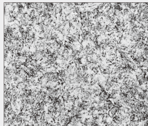
After quenching tempering (x 400)
